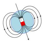
Magnetic Lines of Force: The magnetic field of a magnet is the boundaries of its magnetic lines of force. These are the north to south lines in a magnetic field.
