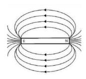
Magnetic Fields: A magnet is an object that attracts certain metals by use of its magnetic field. The space around the magnet contains the magnetic field, which is created by the movement of negatively charged electrons. Electrons have mass, and a slight charge. In magnetic metals, the electrons are unpaired, and spin in the same direction, creating magnetic
